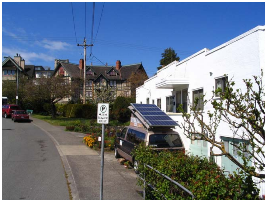
A 3HP (2.5Kwatt) eFarm GT Kit setup on MilFORD the Van at TQELX.COM. (Wind Turbines & GT inverter plant not shown here)
